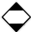
Limited Quantity Ground
